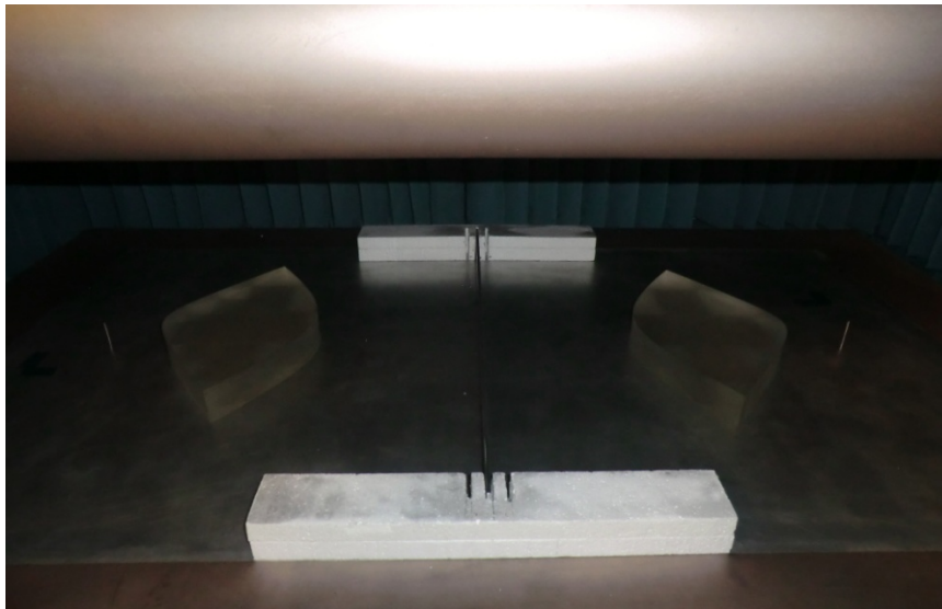
Figure 56 Large lens measurement set-up. The left monopole is connected to port 1 of the PNA and the right monopole is connected to port 2 of the PNA.
