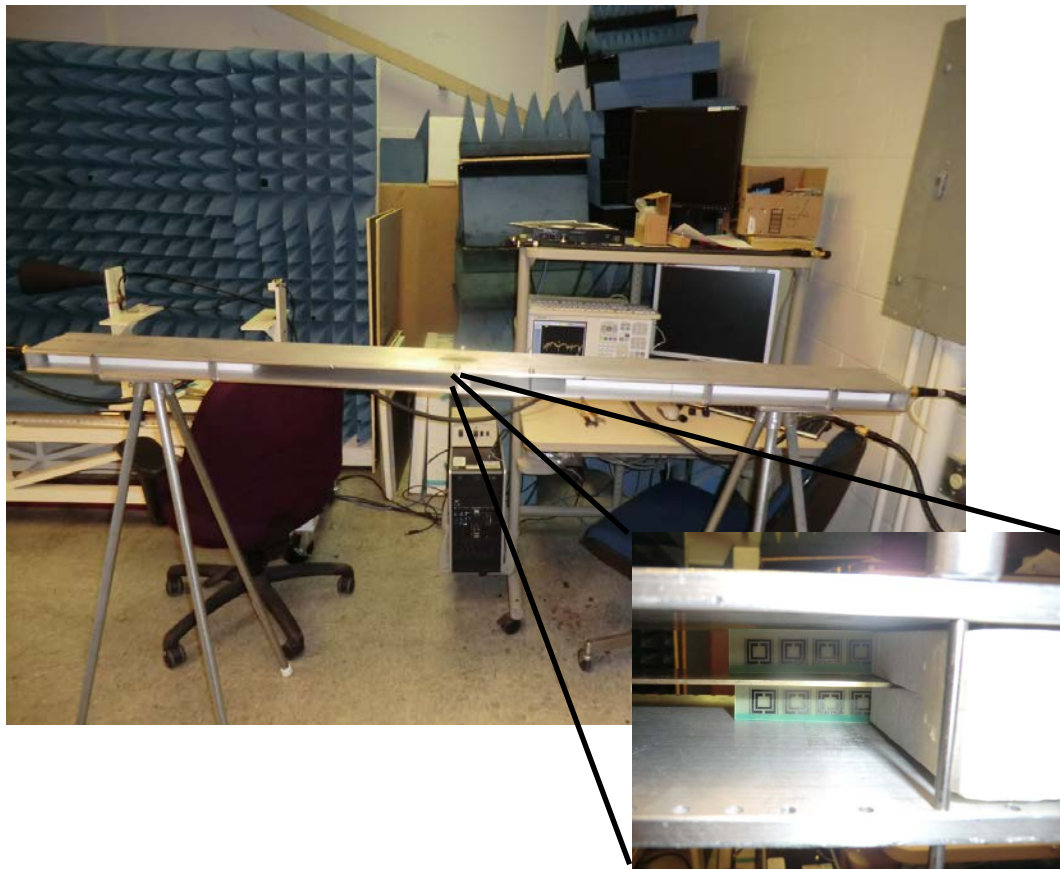
Figure 12 0-4 GHz Stripline used to measure 1-D metamaterial samples and close-up of sample measurement set-up.
