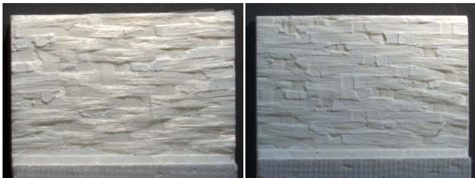
Figure 25. Fracture surface of the DNS specimen tested in compression to failure at 1100 °C in air (test duration < 15 s).
