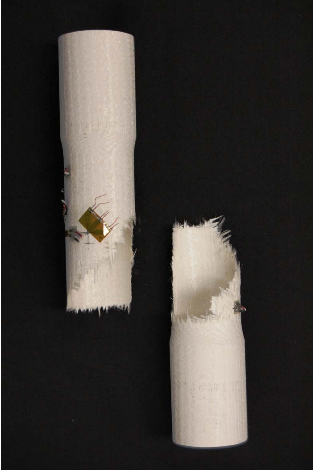
Figure 38. N720/AS specimen B tested in combined tension torsion with the SR of 1:1.
