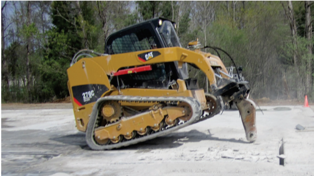
Figure 9. Caterpillar CTL279C with the H65D S hammer attachment.
