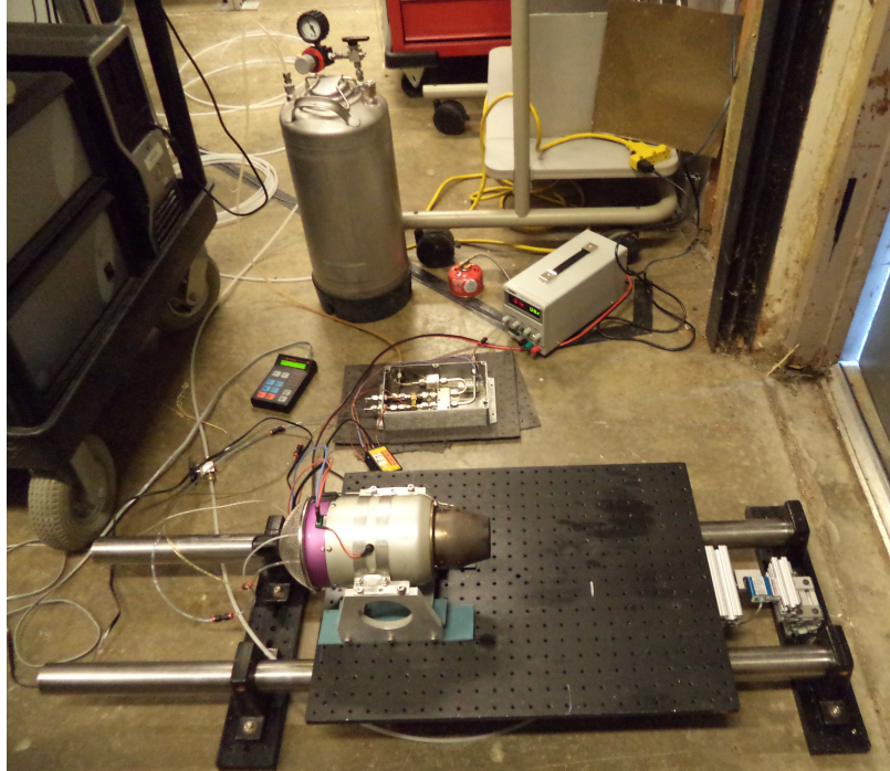
Figure 61: JetCat P200 on Thrust Stand
