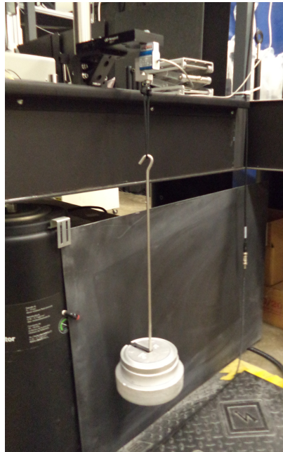
Figure 64: Force Transducer Calibration Setup
