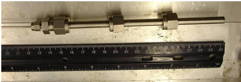
Figure 2.14: Open-ended feed tube/shroud combination injector [24]
