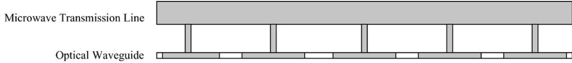
Figure 2.8: Segmented traveling-wave electrode design, showing the microwave transmission line along the top, and the optical waveguide and modulation sections on the bottom. [52]
