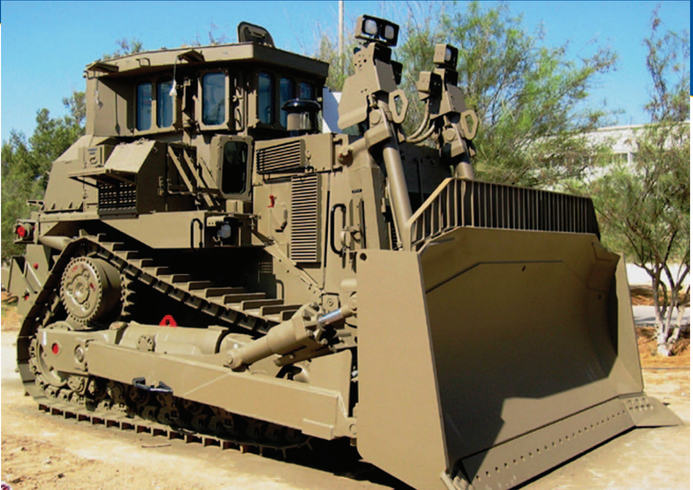
Obtaining Technical Data Packages used to manufacture spare parts allowed DLA Land and Maritime’s value management team to increase competition when procuring parts for up-armored construction equipment, like this heavily armored Caterpillar D9 bulldozer. Previously bought sole-source, the competitive technical data packages have led to a total of $1.6 million in savings to date.
