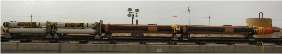
Figure 1: Four Stage Rocket Sled Apparatus. [37]
