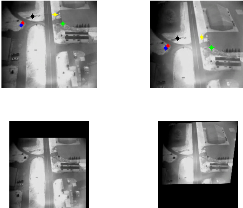
Figure 50: SWIR test flight imagery with feature point matching applied for projective transformations and image registration. Top left, first 1050nm frame with feature matches indicated by the colored points. Top right, original image from next 1050nm frame. Bottom left, first frame with projective transformation applied. Bottom right, second frame with projective transformation applied.
