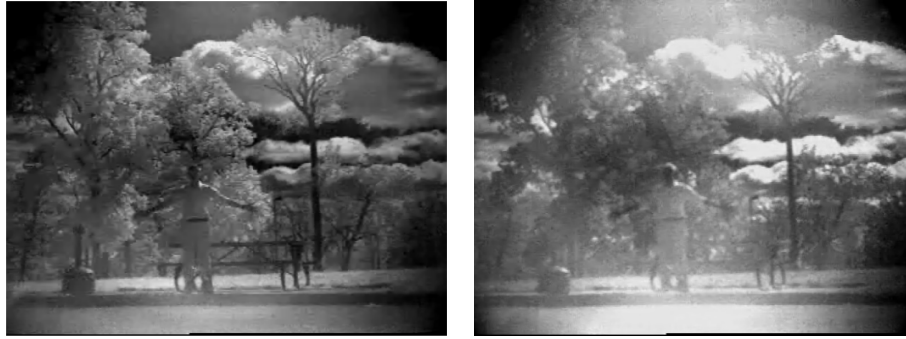
Figure 58: Ground test images. Left is 1050nm in focus, Right is 1550nm out of focus.
