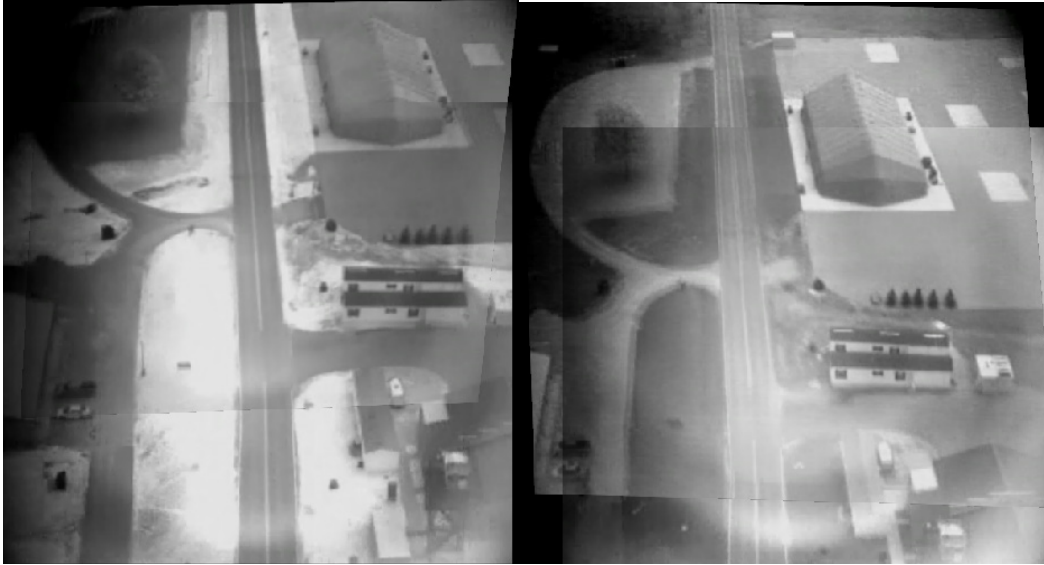
Figure 51: Left, 1050nm video frame, after projective transformations applied. Right, 1550nm video frames
