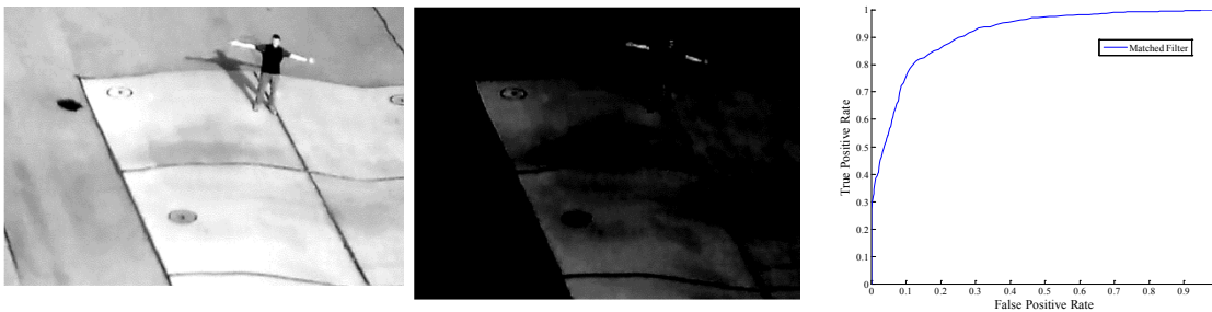
Figure 56: SUAS MSI flight test detection example. Left, MF score from VIS Bands. Middle, MF score thresholded. Right, ROC Curve with resulting AUC = 0.9118
