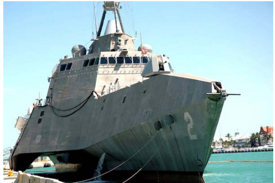
New generation Littoral Combat Ship (aluminum triple-hull combatant) for US NAVY
