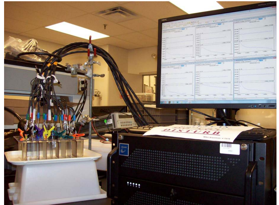
8-channel potentiostat for simulated pitting under galvanic influence
