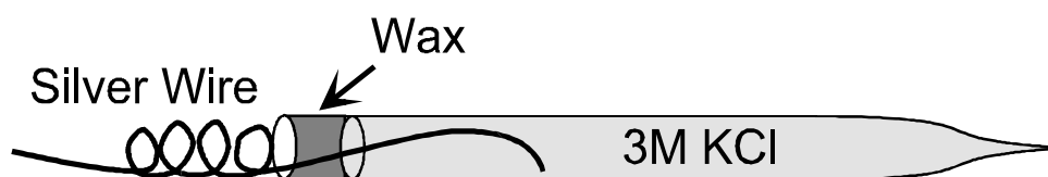
Figure D.1: A drawing of a microelectrode. A microelectrode is a glass pipette with a sharp tip (approximately 1\mu\text{m} in diameter). It is filled with a 3M KCl solution. The solution is contained and the silver wire is held in place by some wax placed in the end.
