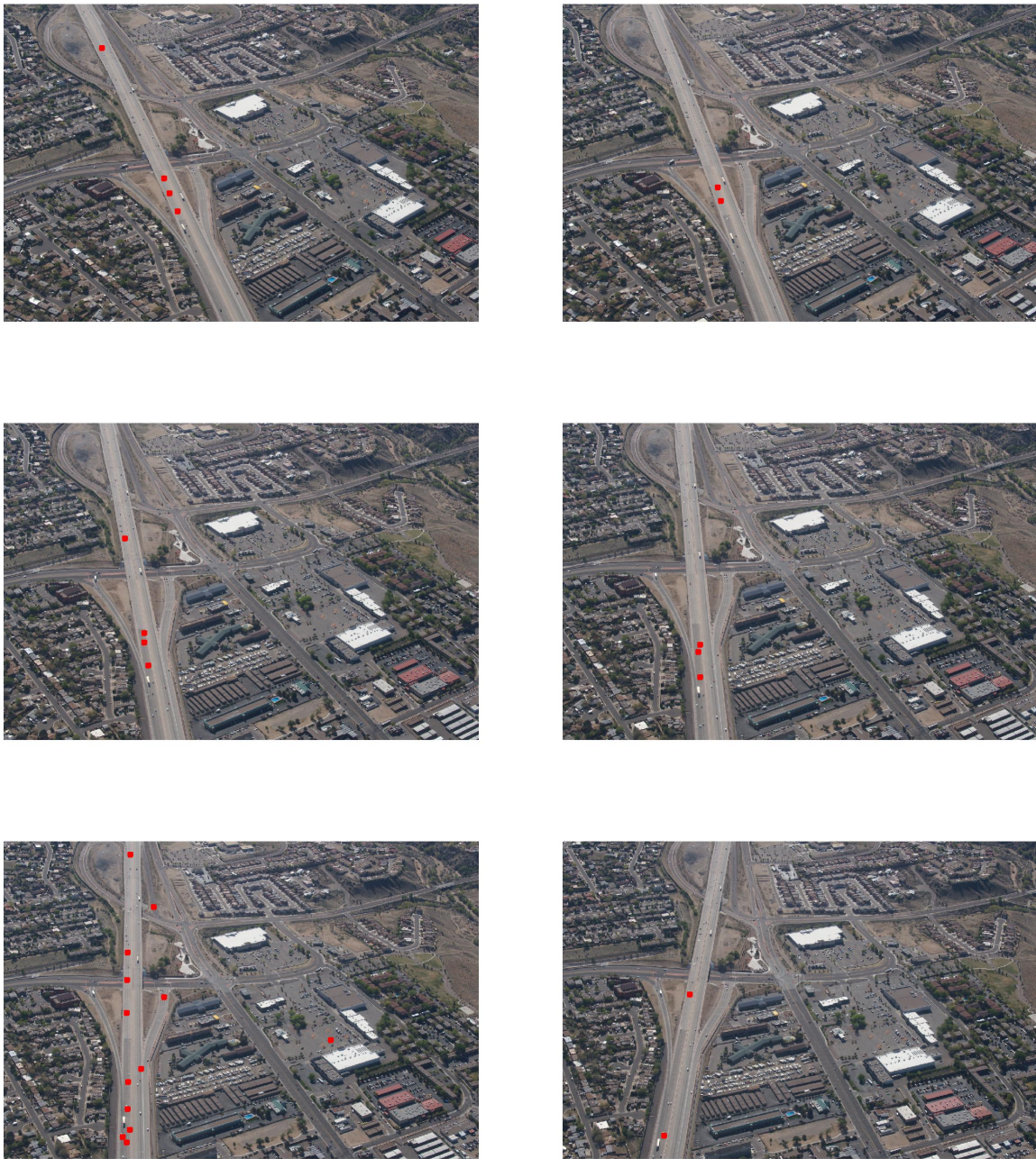
Figure 3.2: Example of LOFT detection on 14 successive frames using a template initiated by an operator
