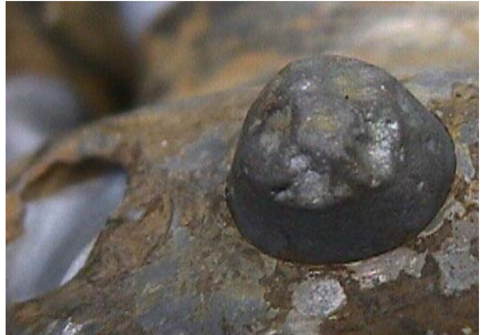
DC carbide rock drilling insert survived severe damage. No catastrophic breakage.
