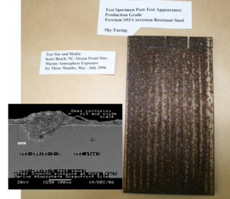
Exposure tests at QuesTek (left) and Kure beach (center, right)
