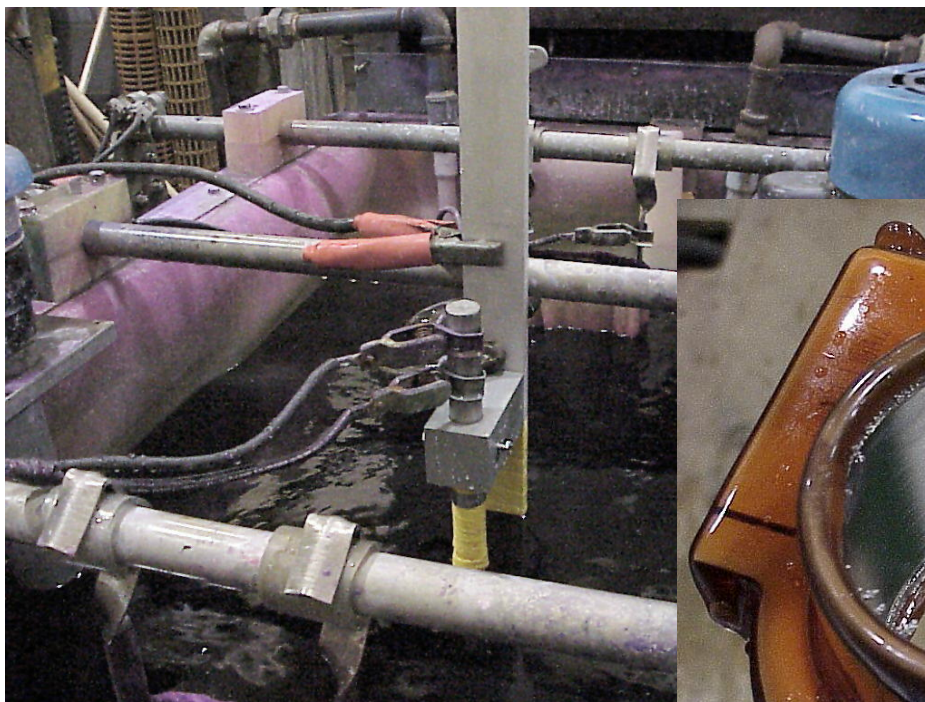
nCo-P Plating on ID: Section from P-3 MLG Actuating Cylinder
