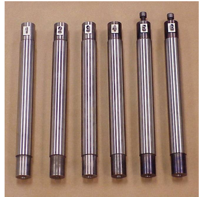
Four 4130 and two 15-5PH rods used for pre-grinding study
