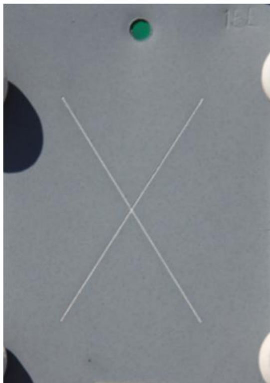
Chromium spray primer over Cr conversion coat 10 rating
