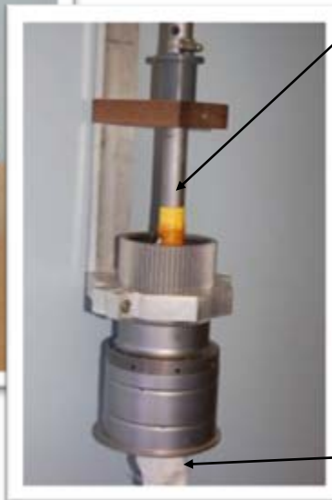
J-52 Coupling, Turbine Shaft Material: 4340 Steel (AMS 6415)
