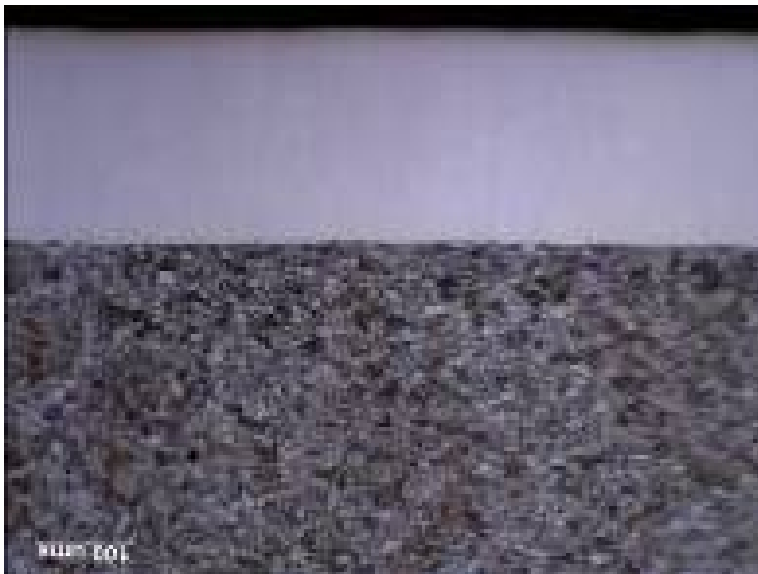
Cross section of nCoP deposit. No pits, cracks or pores.
