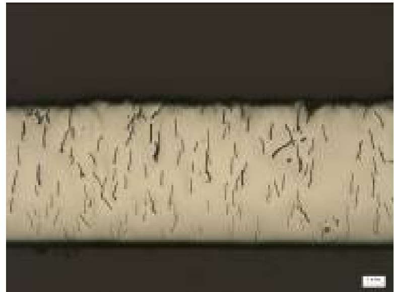
Cross section of EHC deposit. Microcracking observed.
