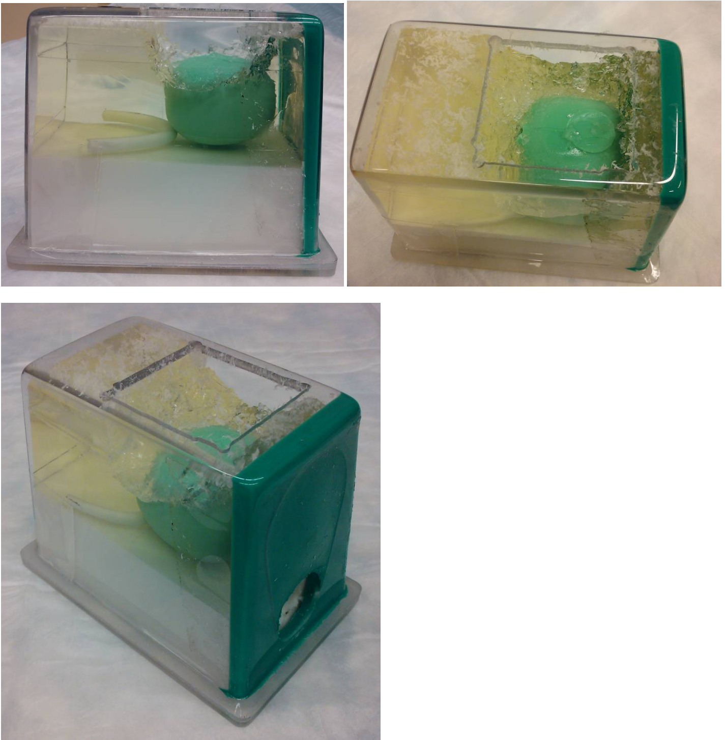
Figure 5: Modified CIRS 066 Prostate Elastography phantom. The top has been removed and direct access to the prostate-mimicking tissue was made available.
