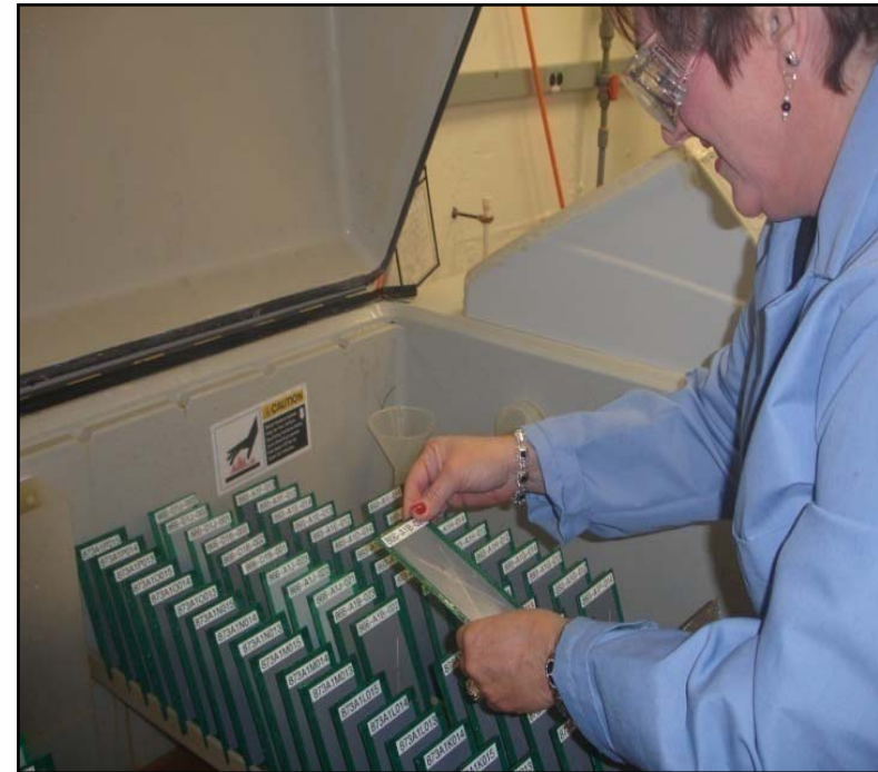
Technician loading test panels into salt-fog (salt spray) test cabinet (ASTM B117)
