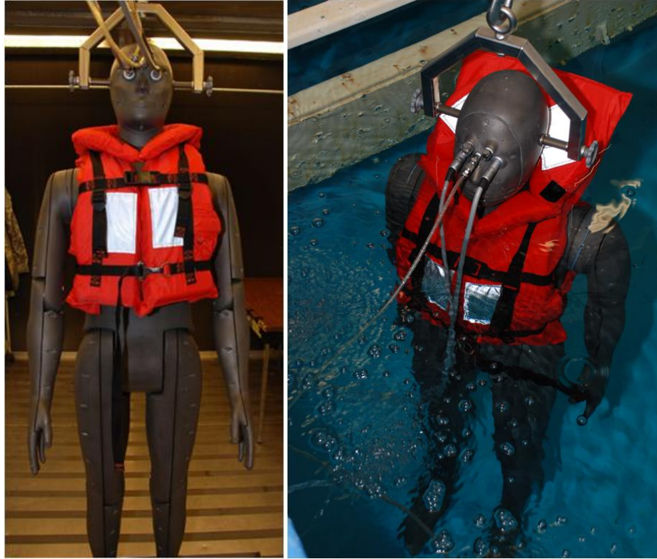
Figure A1 Nemo in climatic chamber (left), and water tank (right) with Stearns Type I PFD
