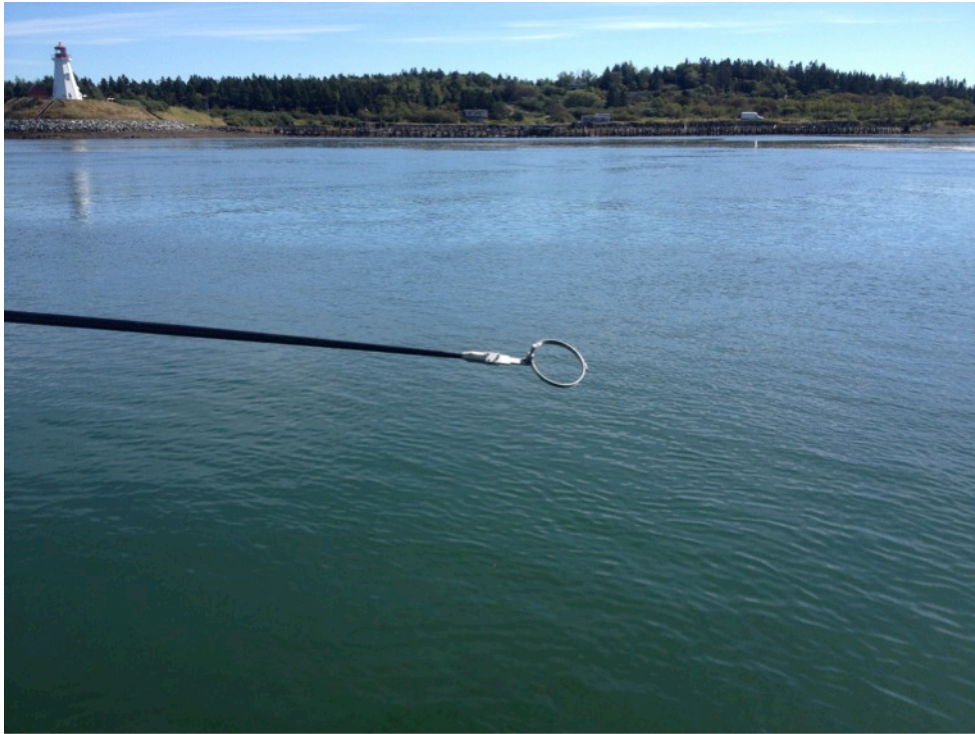
Figure 1. "Hoop" style sampler in close-up (top) and attached to pole (bottom). A nylon veil can be stretched across the stainless-steel hoop, and a quick-release pin (visible in top photo) allows rapid interchange with other devices.
