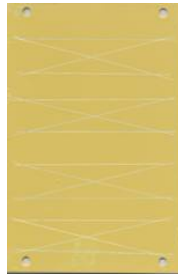
Electroplated Al with MIL-PRF- 23377, after 7 days
