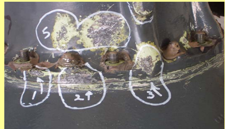
Corrosion on H-53 Tail Gearbox Housing
