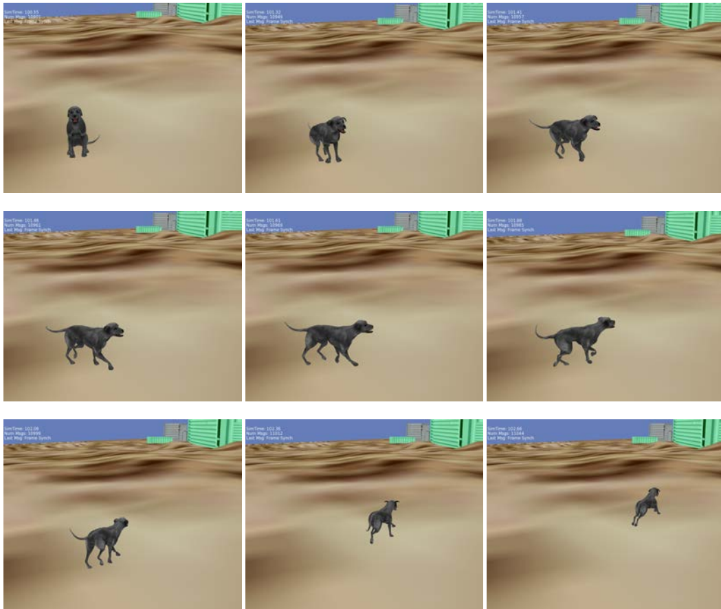
Figure 5: Animation sequence of the “Search” command. Top left: dog in the “Stop” state in the top-level state machine and in the “Sit” state in the animation state machine. Top center: transitioning to a “Search” state in the top-level machine requires a transition in the animation machine to a “Stand” state. Top right: the animation state machine has transitioned to a “Turn” state to orient the dog properly for the “Search” state in accordance with the user command to search in the direction away from the user’s position. Middle row: the dog has reached the “Run” state in the animation machine. Bottom row: the dog accelerates between the left and right images. Animation blending makes the acceleration smooth.
