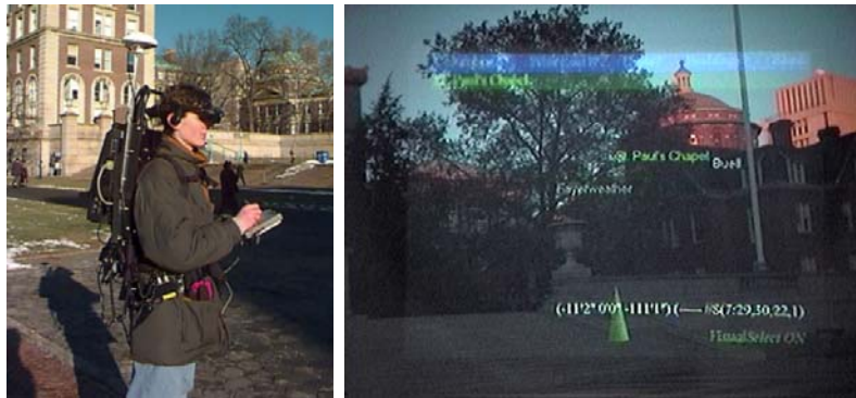
Fig. 1 The Columbia Touring Machine in 1997. Left: A user wearing the backpack and operating the hand-held display. Right: A view through the head-worn display. (Recorded by a video camera looking through the head-worn display.)
