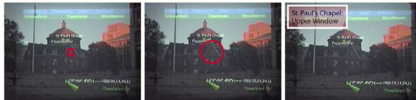
Fig. 6 Left : Accurately aligning a marker on a window can be hard to achieve with tracking errors. Center : A sufficiently large boundary can be guaranteed to enclose the desired object if tracking error is bounded. Right : Text indicators can direct users to the correct point when tracking errors prevent correct registration.
