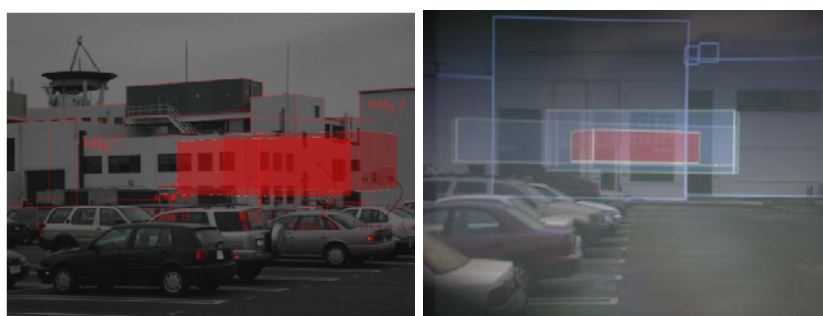
Fig. 7: Left : one of the concept sketches for how occluded buildings and units might be represented in BARS. Right : a photograph taken through our optical see-through display in 2003, with a similar protocol implemented.
