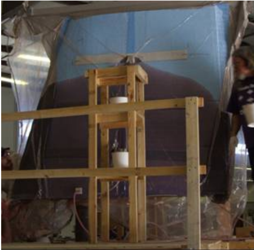
During infusion of first packet (5 layers)
