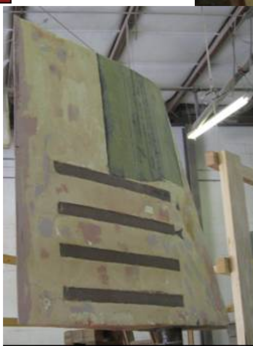
After Infusion of Vertical Shear Ties
