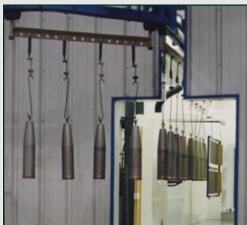
Automated powder application to 105-millimeter artillery projectiles
