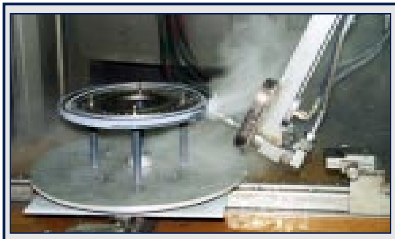
UHPWJ robot removing flame spray coating.
