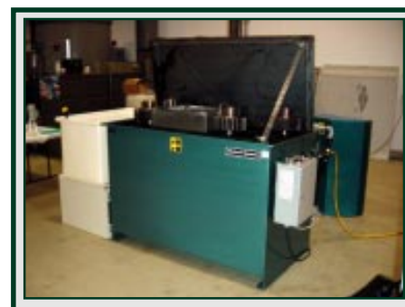
Anniston Army Depot has implemented a lactate esters bath to clean ground combat vehicle components, such as bearings, springs, housings and gears, from engines and transmissions.
