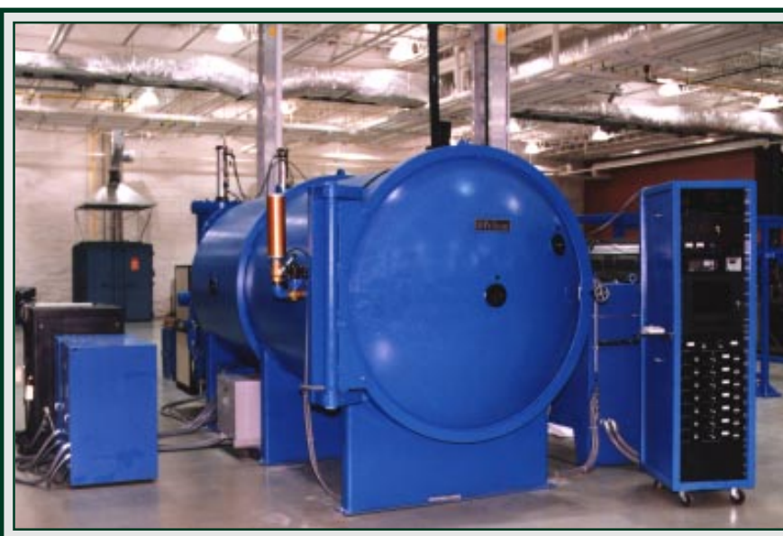
With this PVD technology, components are placed within the chamber and then coated.
