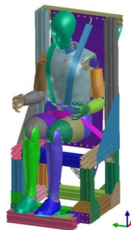
Fig 4. LSDYNA dynamic simulation model including Humanetics v7.1.6 Hybrid III 50th percentile ATD model
