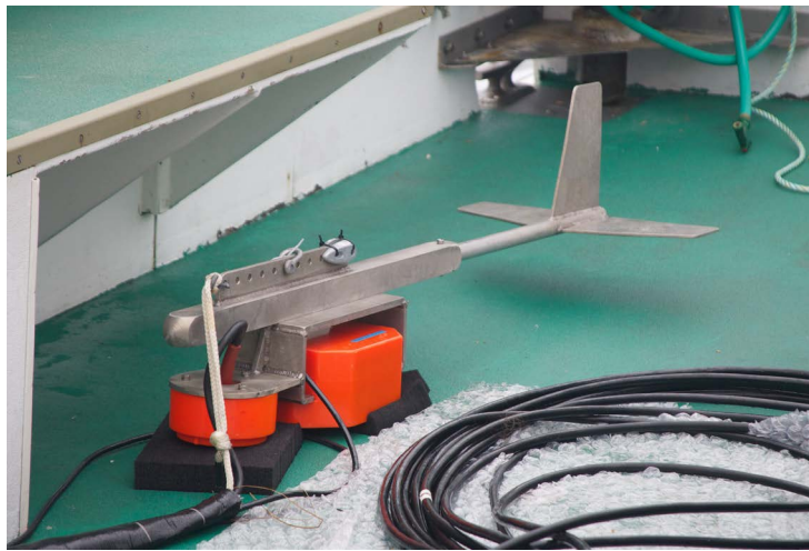
Figure 1. The two echosounder units mounted on the towfish.
