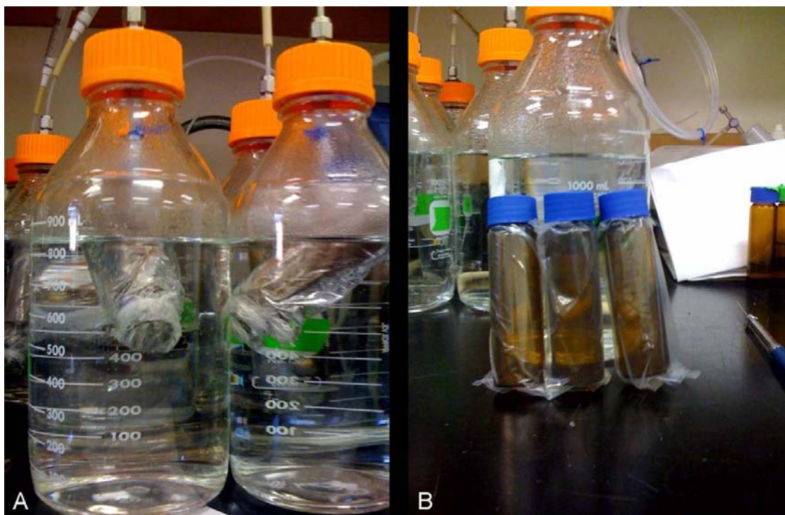
Figure 3.3. Passive vapor diffusion (PVD) samplers and reactors used for passive technique validation. Panel A depicts TCE amended reactors containing the submerged PVD samplers. Double layer LDPE tubing allowed VOC vapor diffusion into the sampler while excluding the penetration of water. Panel B shows the capped PVD samplers after equilibration and prior to GC analysis. 100- \mu l samples withdrawn from the samplers through the cap septa were analyzed by GC.
