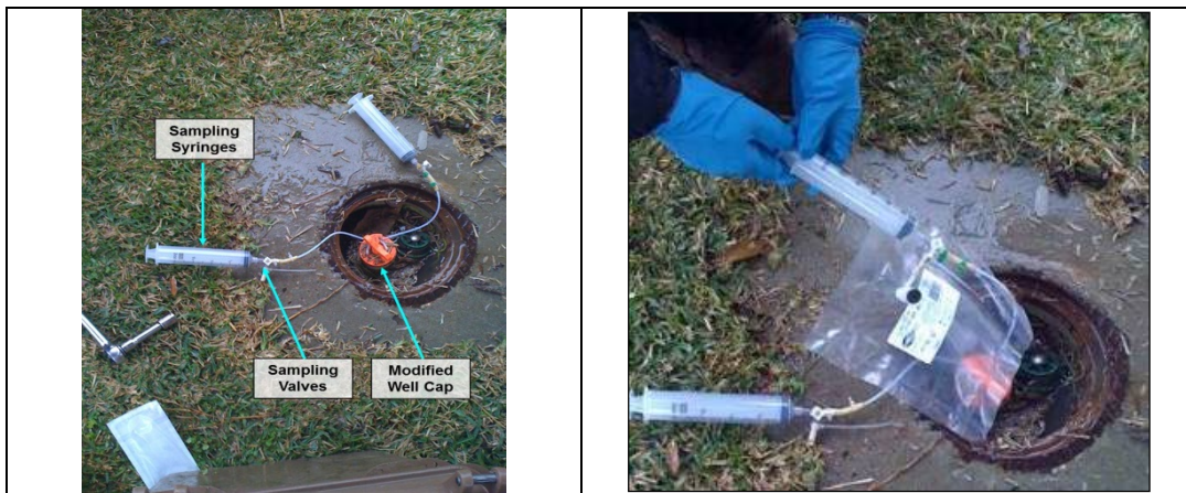
Figure 8. Wellhead sample fittings at a monitoring well for headspace vapor sampling.
