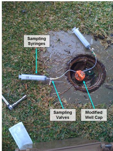
Figure 3.5. Sampling Methods Tested During Preliminary Field Program
