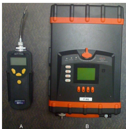
Figure 3.1. Portable field instruments used for the detection of vapor-phase volatile organic compounds. (A) ppbRAE 3000 PID; and (B) Photovac Voyager GC.
