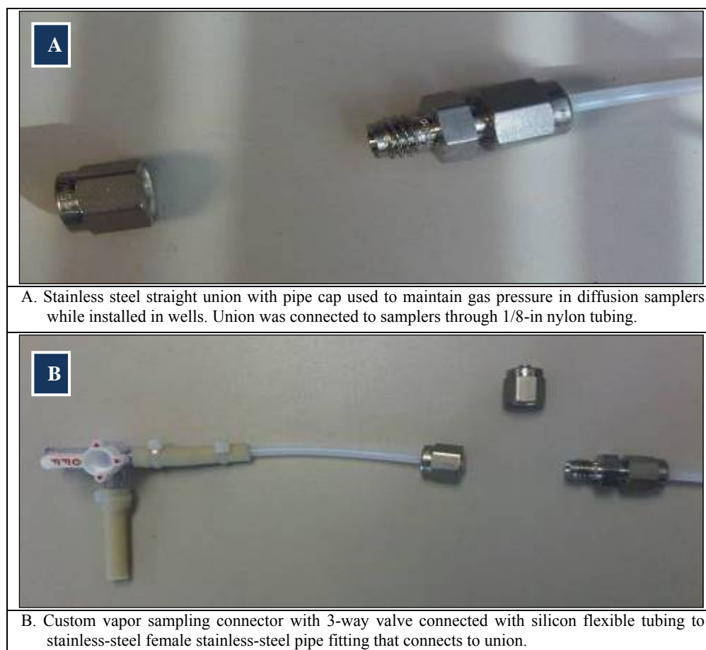
Figure 5. Wellhead sample fittings for extended-length and balloon passive vapor diffusion samplers
