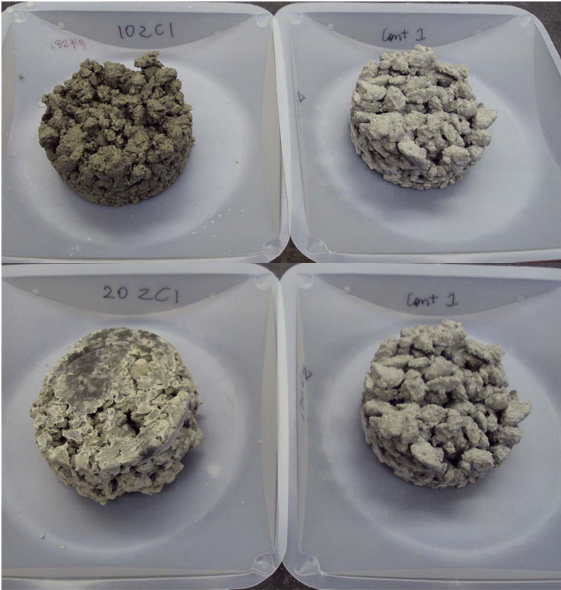
Pictures 5. PAAC with addition of 10 and 20% zeolite clinoptilolite.
