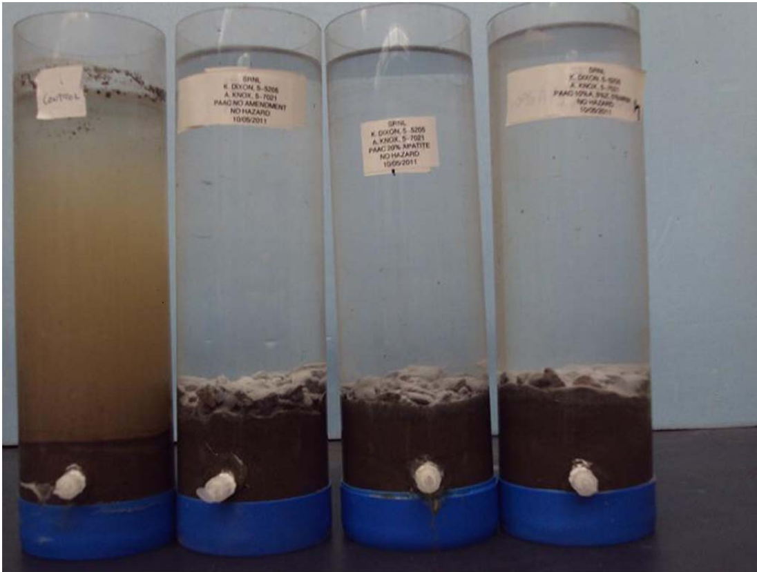
Pictures 2. Columns with two PAAC materials, PC, and uncapped contaminated sediment.
