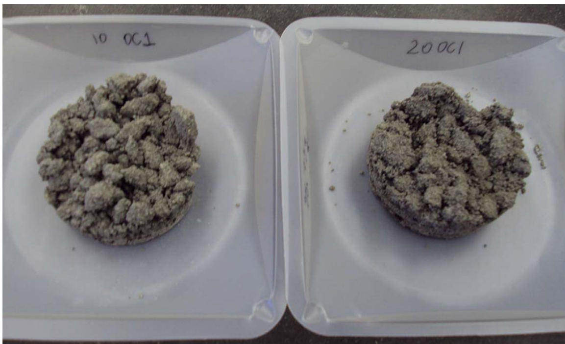
Pictures 7. PAAC with addition of 10 and 20% organoclay (PM-199).
