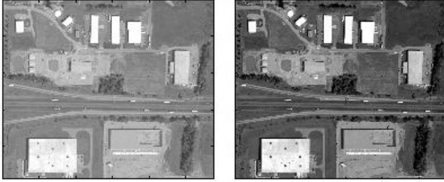
Figure 3.2: (a) The intensity channel of the HSV color model and (b) the image after contrast enhancement. Original image data available from the U.S. Geological Survey [1].
