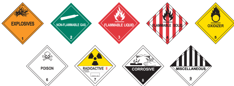
Figure 1: Examples of the Department of Transportation's (DOT) Labels for the Nine Classes of Hazardous Materials (HAZMAT)
