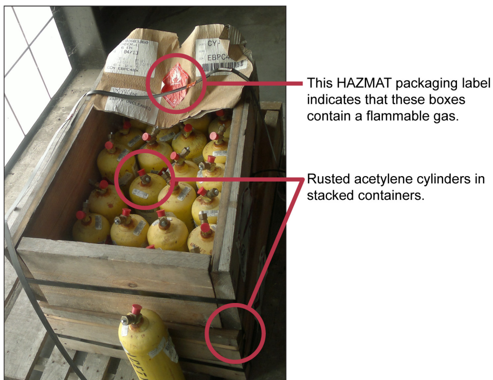
Figure 6: Shipment of Improperly Packaged, Rusted Acetylene Gas Cylinders Delayed in Transport
