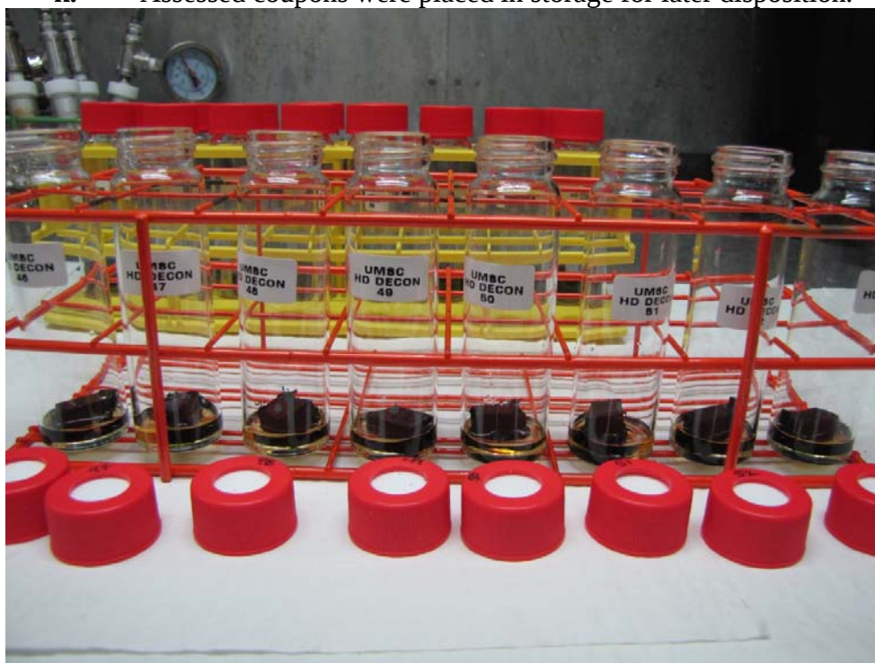
Figure 2. Task 1 coupons spiked with 2 mL of HD for storage.
