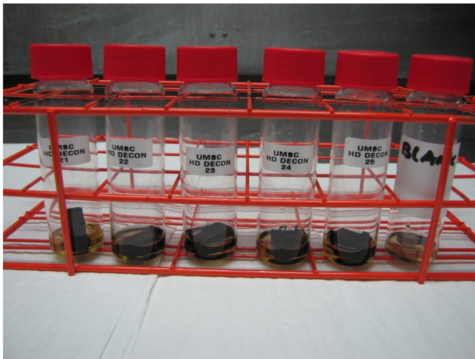
Figure 4. Task 2 coupons and a metal blank spiked with HD before treatment. A metal blank was used in two experiments to verify that the HDPE was not interfering with the reaction between HD and MEA.
