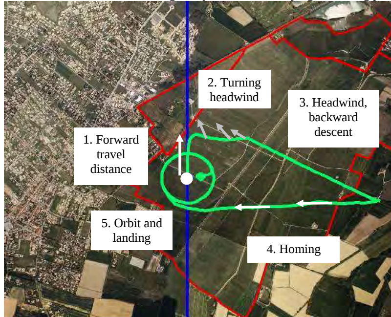
Figure 10 : Top down view of the fast gliding system's trajectory over the CEV drop zone near Toulouse. The Air release point is marked by a white dot.
