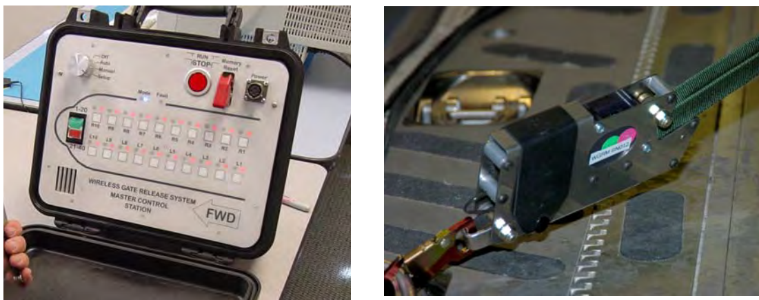
Figure 12. Picture of WGRS MCS (left) and a single WGRM (right)
