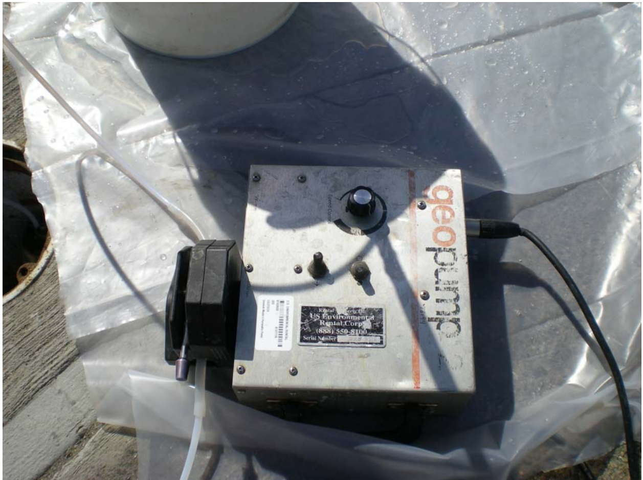
Picture 9. Peristaltic pump for groundwater purging.
