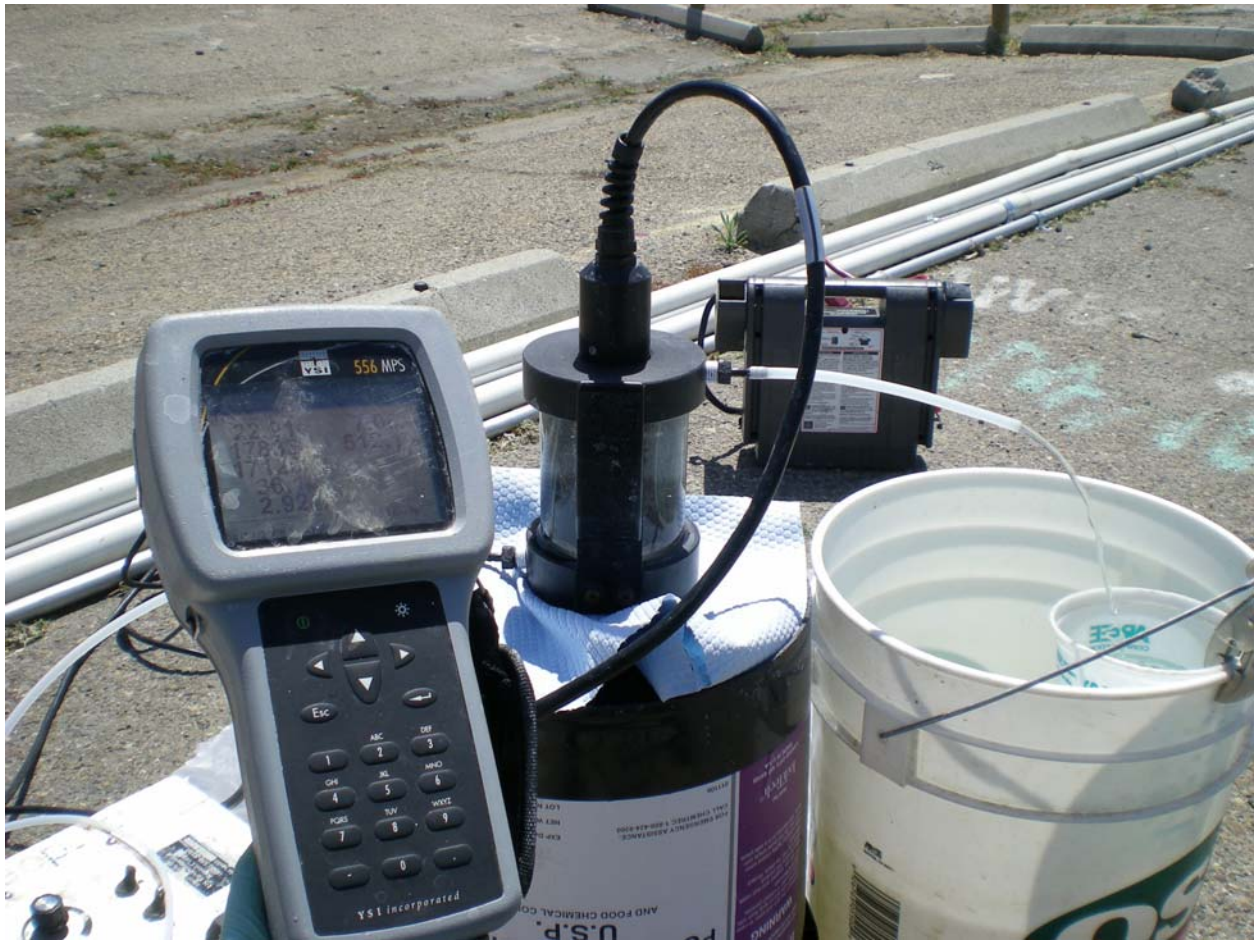
Picture 24. YSI with flow-thru cell for groundwater purging.
