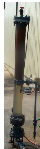
Resin transfer complete. Upper portion of bed still in packed state. Lower portion removed completely.
