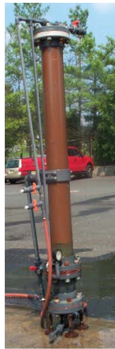
Up- flow applied. Resin is packed against upper header plate. Mid-lateral can be seen on left.
