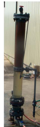
Resin transfer complete. Upper portion of bed still in packed state. Lower portion removed completely.
