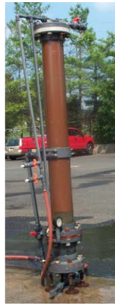
Up- flow applied. Resin is packed against upper header plate. Mid-lateral can be seen on left.
