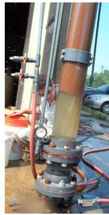
Resin being removed through unscreened mid-lateral.
