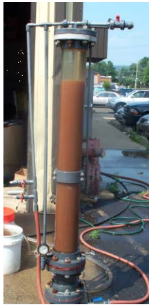
6" Pilot column before flow applied
