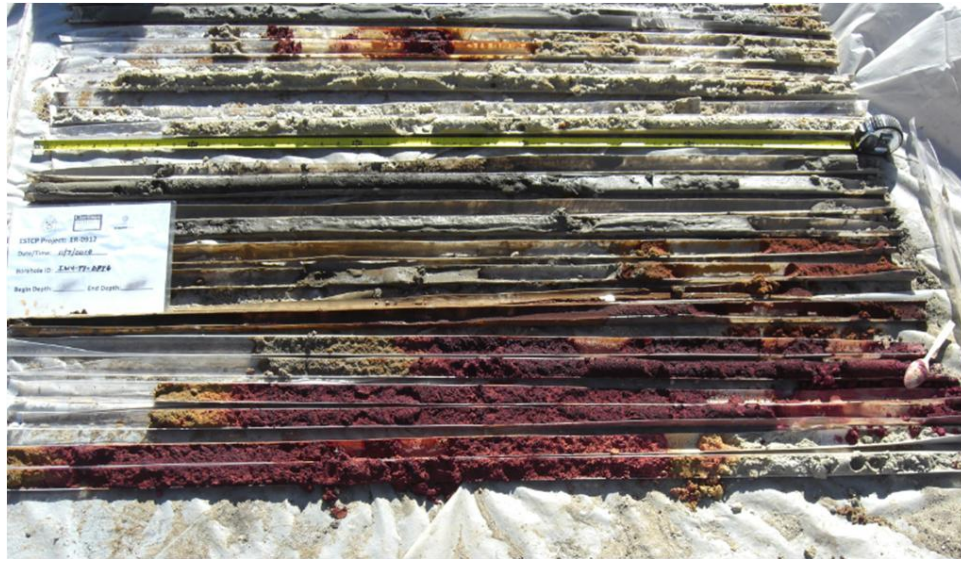
Figure 4. Sediment cores used to vertically characterize the presence or absence of permanganate within the control plot.
