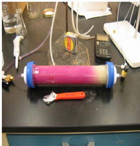
Figure 2-4. Results of 1-D transport experiments for xanthan/KMnO 4 solutions. Xanthan biopolymer transport in clean sand was found to be similar to that of a conservative tracer (i.e., no unexpected retention of polymer).
