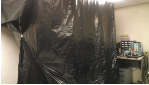
(a) Fully Shrouded Optics Bench
