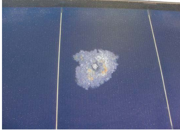
Figure-50: Corrosion of PV material due to a pin-size hole at Site II (NAS Patuxent River).
