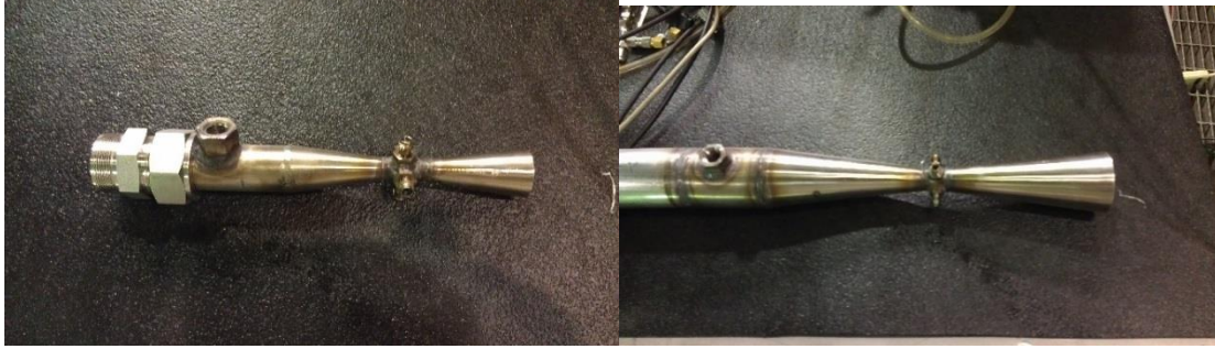
Figure 17: Welded venturis: AO venturi (L) and EO venturi (R)
