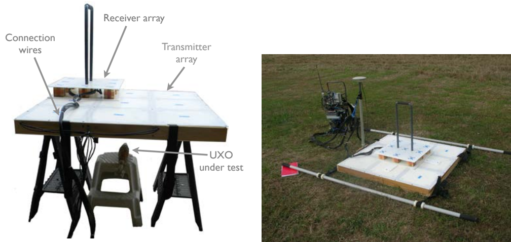
(a) Photograph of the sensor and a UXO under test in a laboratory setting. (b) Sensor in operation at APG on the ground for cued interrogation.
