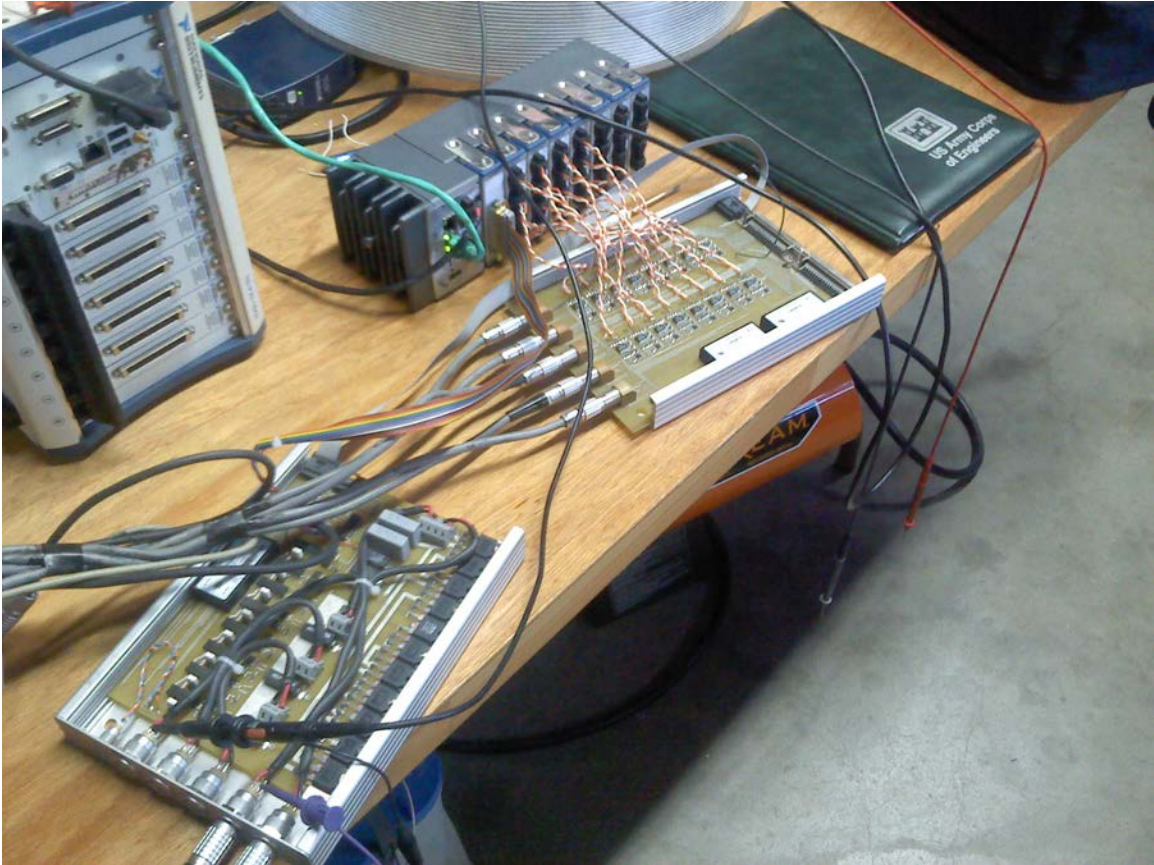
Figure 4.3: Pedemis control electronics. A National Instruments cRIO system with DAQ modules and a digital IO module control Pedemis's transmitters and receivers. See Sec. 4.1.c for more on the electronic control system of Pedemis. The cRIO is programmed in LabVIEW (see Sec. 5.1 for more on Pedemis control software). Also shown are the old transmitter control board (lower left) and the old filter board (in front of cRIO).
