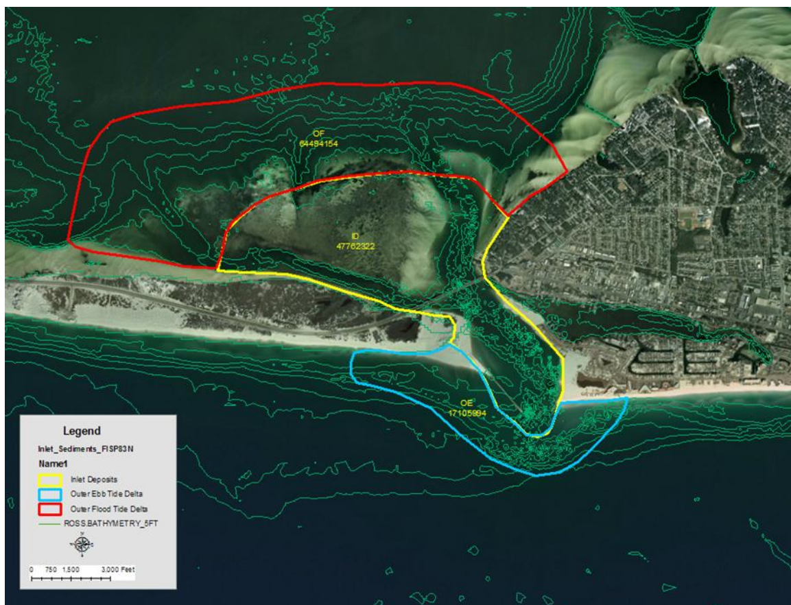
Figure 3.6.2. East Pass Inlet, at the eastern end of Santa Rosa Island, with the areas of the inlet mouth (yellow), flood tide shoal (red) and ebb tide shoal (blue) outlined.
