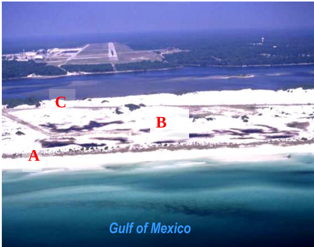
Figure 4.1.2. Northward-oriented, oblique aerial image of Santa Rosa Island near test site A-10. Geomorphic subdivisions visible in the image are: (a) vegetated, 5-meter foredunes, (b) interior stabilized overwash zone and freshwater ponds, (c) stabilized bayside dunes with tree cover. Hurlbert Airfield is visible on the mainland. This image was taken in 1989, before the destruction of the foredunes by Hurricane Opal in 1995.
