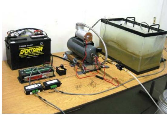
Figure 5.10 Laboratory setup of the air-blast cleaning experiment.
