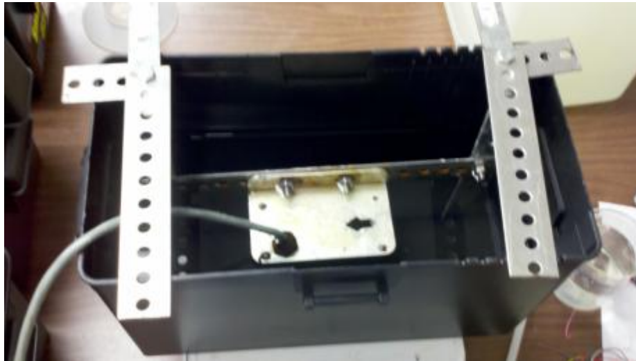
Figure 5.6 Sensor assembly placed in black box (without lid) for pre-calibration in clean water.
