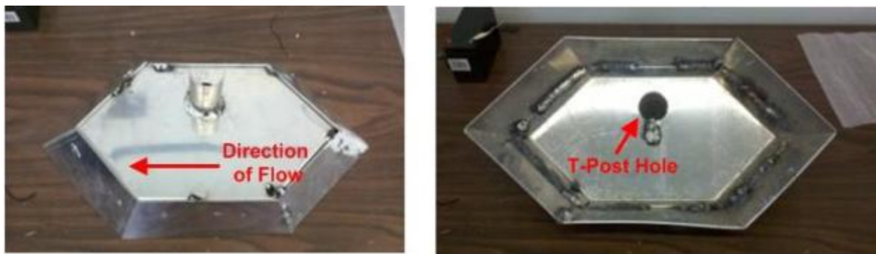
Figure 2.15 Top and bottom views of the new sensor cover design.
