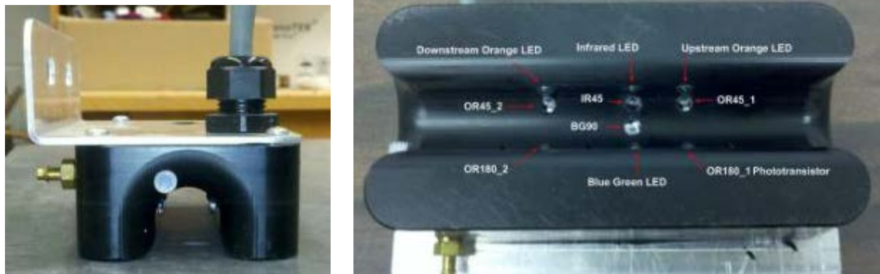
Figure 2.4 Side (left) and bottom (right) views of the Optical Sensor. Note the channel on the bottom of the sensor enclosure.
