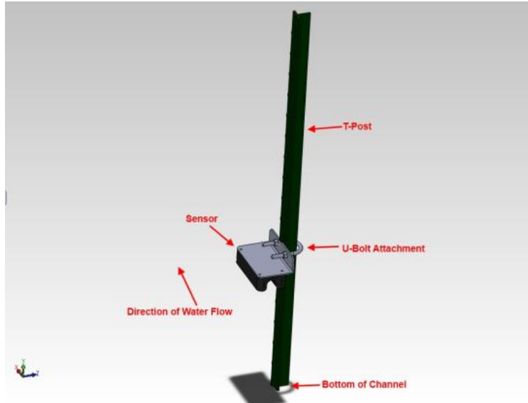
Figure 2.13 Installation of sensor in stream; the sensor is attached to a T-post.
