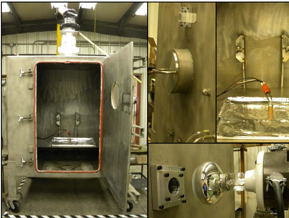
Figure 8: Obscurant 100 cubic foot test chamber {left}, light source for transmittance measurements {bottom right}, light detector, air inlet and gas sampling ports {top center}, pellet ignition system {top right}
