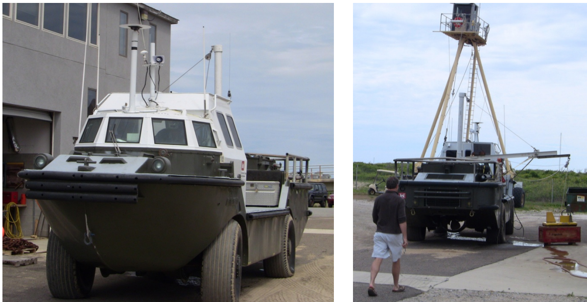
Figure 6 Army Field Research Facility (FRF) Light Amphibious Reconnaissance Craft (LARC)
