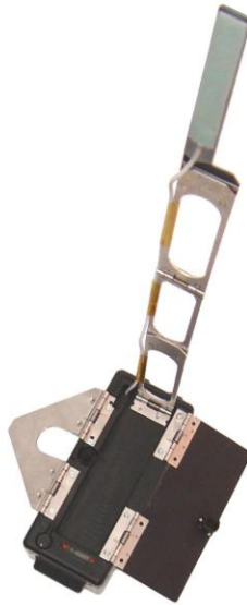
Figure 7. Spring-hinge antenna mast on self-righting relay node.
